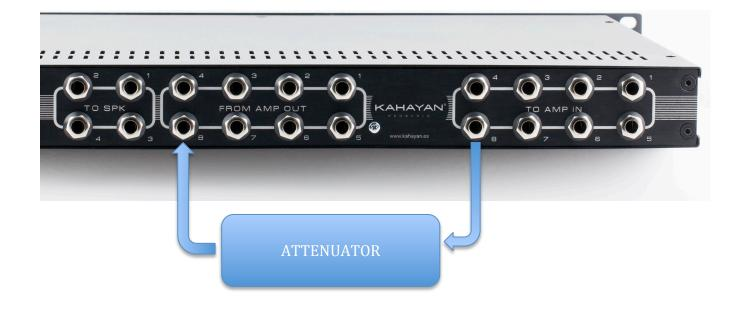
**Working mode 2:** The attenuator works with all amplifiers but only with 1 speaker.
