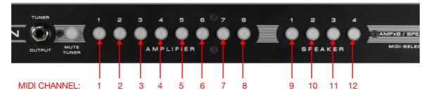
5-Hold the 'MIDI CHANNEL' button you need during a few seconds until the led selected blinks slowly. And hold again the 'Mute' button until you see that this led stops to blink, this mean the new setup is recorded and working.
